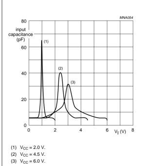
Fig.13 Typical input capacitance as a function of the input voltage.
